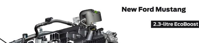
High-flow cylinder head with integrated exhaust manifold moves air in and exhaust out for better performance
